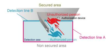
Multiple detection: Generate multiple detection output when multiple people stay in the detection area.
