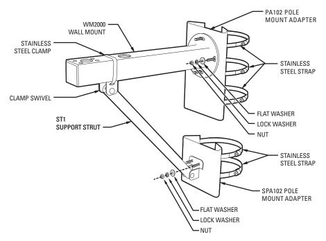
Figure 1. Typical Pole Mount Adapter Installation
