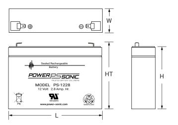
**L**: 5.24 (133) **W**: 1.30 (33) **H**: 3.82 (97) **HT**: 4.09 (104) Tolerances are +/- 0.04 in. (+/- 1mm) and +/- 0.08 in. (+/- 2mm) for height dimensions. All data subject to change without notice.
