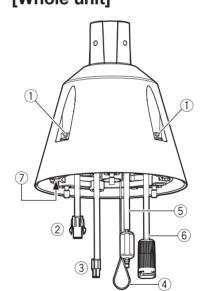
1 Hexagonal socket head special screws (3 positions) Fixes a camera body and this product.
