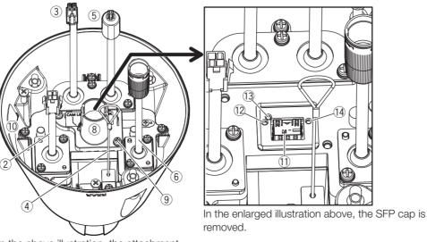
In the above illustration, the attachment ring is removed.
