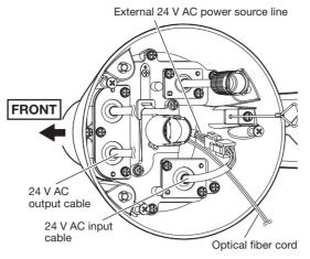
• This product is equipped with two cable connection terminals; one is "24 V AC input cable" that is connected to an external power source cable, and the other is "24 V AC output cable" that supplied the camera with power source. Be careful not to make improper connections.
